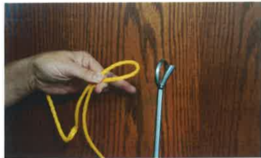
Fig.1 Isolate rope to place Turf Stake and loop
