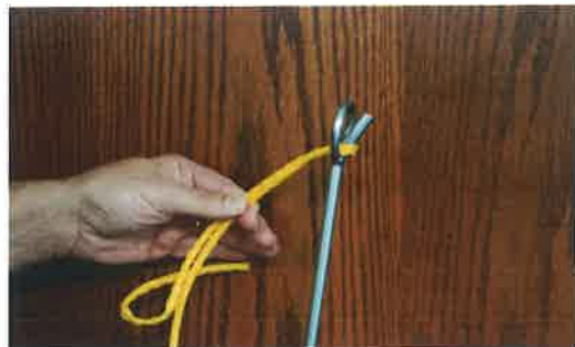
Fig3 Pull the loop down onto steel stub
