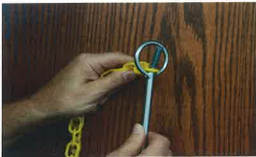
Fig.2 Place chain link through the circle and onto the steel stub
