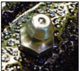
Zerk locations are shown below, and one is also located on the hub of the front tire. Zerk locations are identical on all rear gangs, making 30 total zerks for a five gang, and 20 total for a three gang.
