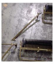
3. On the front gang (with tire) assembly, remove the pin and pin collar from the shaft, leaving the spring as shown in the diagram.
