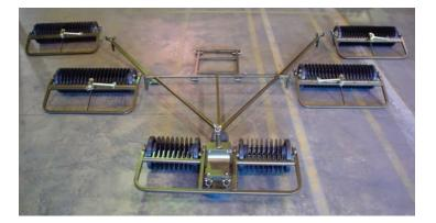
2. Make sure that the right and left arm assemblies are on the correct sides. The correct positions are shown in the diagram to the right. (five gang only)
