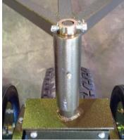
6. Remove the pin collar, and pin from the shaft on the next two gangs behind the front gang.
