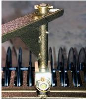
11. Remove the two pins from the rear of the A-Frame. Insert the push frame (as shown) into the space provided. Insert pins and be sure mount is secure.
