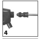
4. Separate the pump assembly by carefully pulling piston from tube
