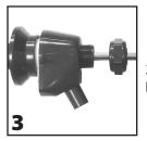
3. Unscrew threaded cap from pump assembly
