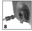
8. Carefully insert piston rod assembly into pump unit
